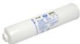
Carbon/Sediment pre-filter for the NEW, #1935-0 Nature's Spring RO unit. This filter contains a coconut shell, activated carbon filter to remove excess sediment and chlorine to extend the life of the reverse osmosis membrane. Easily installed with no tools in just a minute or two.
